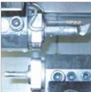
TENDOturn DKE Held in standard VDI boring bars on compact double spindle machines
